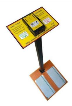
Wrist Straps are the first line of defence against electrostatic charge build up on the human body. This instrument is designed for fast, frequent testing of ESD wrist straps and Footwear. It is very simple to operate. A green light signals the user that everything is OK. A red light and an audible indicator means that the circuit resistance is either too low or too high.
